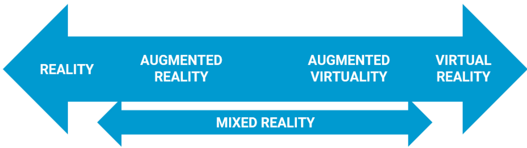
Fig. 1. Milgram's reality-virtuality continuum is a continuous scale ranging between reality (no synthetic imagery) and virtual reality (only synthetic imagery). Between the two ends of the continuum is mixed reality , where real and synthetic imagery are combined with either synthetic imagery added to a real environment as augmented reality or real imagery added to a synthetic environment as augmented virtuality [59].
