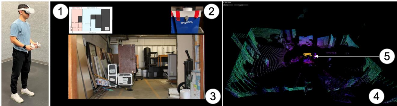
**Figure 3:** (Left) users wore a virtual reality HMD and two handheld motion controllers. (Middle) [1] warehouse floor plan, [2] image of the target search object, [3] real-time 3D stereo video stream. (Right) [4] real-time 360° dense point cloud, [5] state visualization virtual robot of the Spot embedded within the 3D reconstruction.
